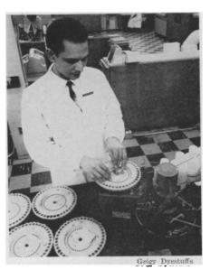
COLOR COORDINATOR—Color matching for textile industry can now be accomplished by a computer that can also calculate the precise amounts of dyestuffs needed to produce an exact shade requested by a designer. Chemist Robert St. John uses the computer on a cloth sample to break down mathematically the shade into its components at Geigy Dyestuffs, a division of the Geigy Chemical Corporation, Ardsley, N.Y.
