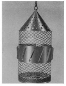
cage-like device that scales the fish as they are dragged along in it behind the boat. Designed with a perforated metal nose cone and a circle of diagonal fins around its center, the scaler rotates as the water passes through it. The scales are removed as the fish are shuffled against the wire mesh and the water passing through washes them away. The unit also serves as a holder for the catch.
