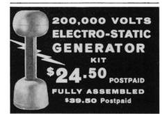
200,000 Volts, as illus., can be assembled with pliers and screw driver. 17" high, 7" diam., Current 1.5 to 2.5 microamps. 90% rel. humidity range. Life of service over 1000 operating hours. 110 v 60 cycle AC motor, insulating column of unbreakable vinyl chloride, oil impregnated bronze bearings. Aluminum base, housing, frame and charge collector — 5 lbs.
