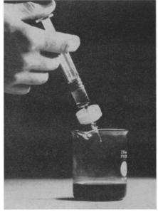
SYRINGE FILTER HOLDER, shown in photograph, for membrane filters, fits any standard syringe. Suitable for use in filtering small volumes of liquids, the filter holder is made with autoclavable plastic and a stainless steel filter support screen. Attached to any wash bottle it provides membrane-filtered particle-free water. The holder is also useful for in-line filtering of air.
