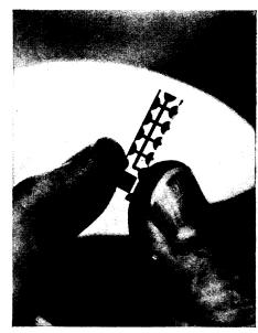
**EXPERIMENTAL DIODES—Scientists at** International Business Machines Corporation have discovered a new type of tunnel diode having "negative resistance." An array of experimental MOS tunnel diodes is shown. The longitudinal line is an oxidized aluminum strip and the perpendicular lines are strips of tin telluride. Each intersection forms an MOS tunnel diode junction.
