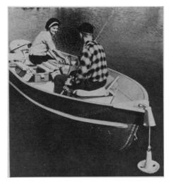
ANCHORING DEVICE, shown in photograph, is a 4½-inch diameter reel that can be mounted at any convenient spot on the boat. Designed for small boats, the device allows one-hand control of the anchor from a sitting postion eliminating the need to move about or stand to raise or lower the anchor. The bow mount which comes with the reel holds the anchor away from the boat preventing it from bumping the hull.
