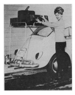
LUGGAGE CARRIER for Volkswagen sedans, shown in photograph, allows full rear vision for the driver. Built of lightweight tubular aluminum, all - welded frame construction weighing six pounds, has a ninefoot platform and loads up to 15 pounds. Its rear legs attach easily to the rear bumper and can be locked securely to the sedan.
