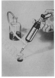
PIPETTING GUN, shown in photograph, operable with one hand can be set to dispense liquids at a preset amount at any volume from 2 cc to 30 cc indefinitely at an accuracy within plus or minus one percent. Its stain-less steel barrel is Teflon coated and free from sticking or freezing. The gun is easily cleaned, chemically inert and autoclavable. The unit comes complete with tubing, check valve and sinker.
