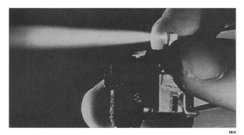
LASER LIGHT—A process for making an injection laser was patented by International Business Machine Corporation. The photograph was taken with infrared film, since the laser emits infrared light with a wavelength of about 9,000 Angstroms. The laser shown emits pulses of light of about 10 watts at room temperature.
