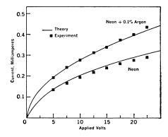
Characteristics of tubes filled with gases ionized by fission fragments. Resulting current is a function of ion generation rate, which is increased greatly (from 1.8 to 2.6 x 1016 ions per cm<sup>3</sup> per sec) by small addition of argon,
