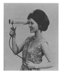
VIEWFINDER TV CAMERA, shown above, 10 inches long and 3 inches in diameter, is especially useful for taking fast-moving events such as sports, dramatics and scientific phenomena. Weighing only three pounds and easy to use, the camera has a fold-away handle with an on-off trigger that remotely controls equipment, such as a video tape recorder, monitor or receiver, connected to it. The device operates on silicon transistors.
