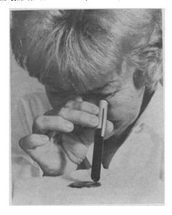
COMBINATION TELESCOPE-MICROSCOPE, shown in photograph, clips in the pocket like a fountain pen. It is a single unit device that can be used to observe tiny biological specimens as well as the stars in the heavens. Useful to students as well as homeowners, campers and bird watchers, the instrument consist of an 8x power telescope and 30x power microscope. Six inches long and 5% inch in diameter, it can be kept conveniently at hand.
