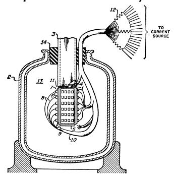
Solid state crystals are one common source of laser beams. Usually the crystals are excited by radiation from gas discharge lamps, which are inefficient, cause heat problems and don't match the frequency of light put out by the solid state crystal.
