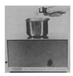
This compact table-top ultrasonic unit for laboratories operates at a frequency of 22 kilocycles per second and is suitable for routine cleaning as well as for degassing solutions, decontamination of slides or nuclear glassware. Convenient and simple to use, and provided with an automatic shut-off to prevent overheating, the cleaner is self-tuning for solvent level, temperature and nature of the object being cleaned.
