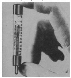
by-1/2-inch instrument will measure shock from 5 to 100 g's when taped to the object to be tested. Easily set and reset, several of these units can be attached to equipment or packaging to test maximum force from various directions.
