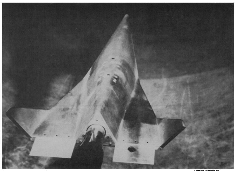
HST designs can see into the future in this high-speed test tunnel, which blasts them with air at up to Mach 20.
