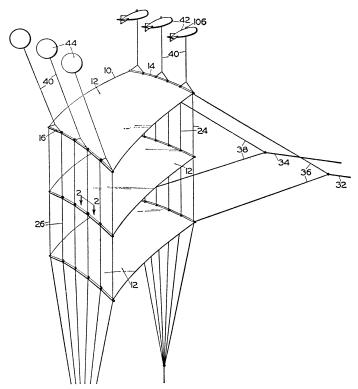
structure would be relatively streamlined, so that air would push more strongly against the rear balloons, keeping the package facing in the proper direction.
