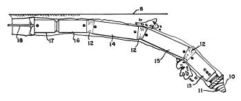
impenetrable obstacle such as a big rock. If its power supply is cut off by accident, an emergency power unit sends the gopher up to the surface.
