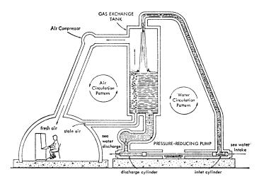
The surfaces of the many droplets and bubbles act as diffusion membranes. The excess carbon dioxide in the stale air diffuses into the seawater, and the oxygen in the seawater diffuses into the air. The revitalized air is returned to the living chamber of the structure.
