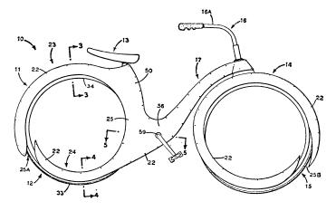
fender-like frame. Rubber mounts between the rollers and the frame take the road shocks that in conventional bicycles are absorbed by the tires.
