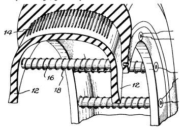
has rods that fasten to pins on the wheel rim, eliminating the slip-off problem.
