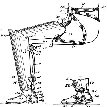
Even the man-sized units, however, are so heavy that they have been designed with wheels or skids at the bottom to support part of their weight. In addition, an elaborate system of straps distributes the weight of the armor around the wearer's body. The armor might be made of steel or titanium alloy and should withstand velocities of at least 2,800 feet per second for .30 caliber "ball and antipersonnel projectiles," says the inventor, who assigned rights to the Army.
