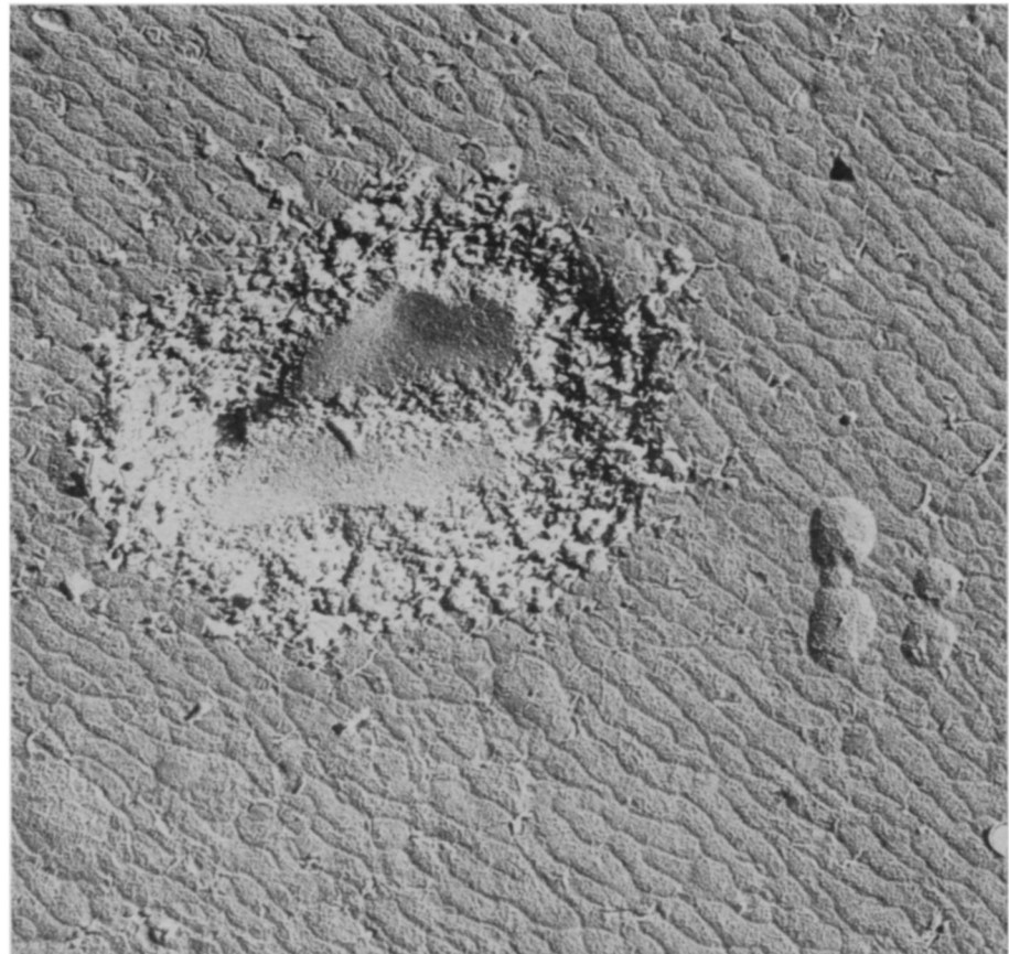
Tiny spot in aluminum alloy succumbs to corrosion faster than the rest.
