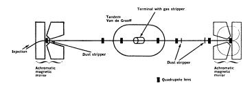
will acquire on the average a greater positive equilibrium charge than ions passing through a gas stripper, the kind normally used in a Van de Graaff accelerator.
