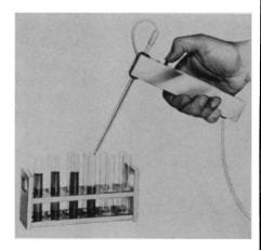
two syringes and an electromagnetic check valve, the unit, which mounts on a side of a cabinet, dispenses a preset volume of sample with a preset volume of diluter directly into the test tube.
