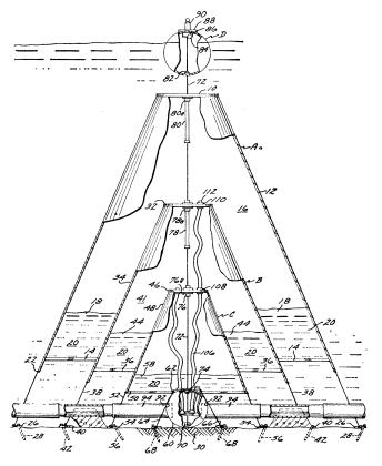
unit that consists of a series of cones, stacked points-up. The unit would only be used for substances, such as oil, that are lighter than water, so the cones would have no bottoms, and would simply be tied down on the ocean bottom, one above the other. Water pressure would keep the chemicals up inside the cones.
