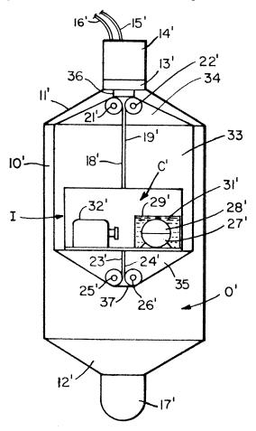
forces can be enough to counteract the capillary action that keeps the fuel flowing when the rocket motor is firing. This is the problem being studied by the Martin-Marietta Corp., three of whose scientists have just been granted a patent for their unique free-fall test facility.
