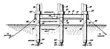
An invention patented last week attacks the problem of heaving platforms directly by putting propellers on the ends of the supporting pillars. Motion sensors in each pillar sense when that part of the platform is moving up or down and drive the propellers to counteract it.
