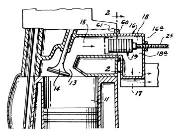
cylindrical insert in the exhaust manifold of the engine. The metal insert retains the heat of the exhaust gas as it comes out of the cylinder and slows the gases down so that more complete burning takes place.
