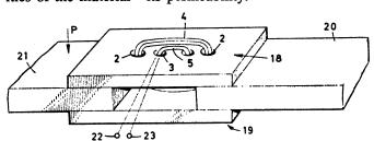
If a force is applied to the material, its permeability changes, and the measured voltage changes with it.
