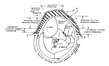
Van Patten of Wright-Patterson Air Force Base, Dayton, Ohio. Most of the discomfort, he adds, is concentrated in areas where there is relatively little body tissue between the restraint and the astronaut's bone. A prime candidate is the lower leg.
