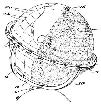
with the earth's rotation. Around the globe's equator is a band which is engraved to show the 24 hours of the day. To find the time at any place a user reads the hour and minute mark under which its meridian of longitude is momentarily passing. If the globe is made translucent. a partial shadowing shell inside it can be used to indicate night and day.
