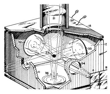
particle will change its position. Photoelectric sensors note the shift and actuate a servomechanism that adjusts the electric field until it balances the new force and the particle returns to center. The amount of the acceleration can then be determined from the changes in the field.
