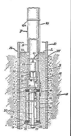
ered into a well; the cylinder is about half the diameter of the well casing, its length equal to or greater than the diameter of the well.
