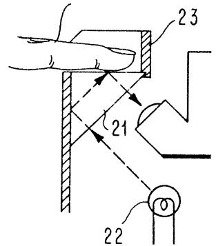
In the invention patented by Claus H. Claassen and Louis D. Green, an identification card contains a magnetic tape record of the pulse pattern produced by the card-holder's fingerprint. When he is to be identified, the system compares the pattern stored on the card with the pulse train produced from scanning his finger. If the two patterns are the same, the identification is made.
