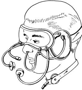
The movements of the lips, for instance, are sensed by transducers, which produce a waveform that can be reliably identified by a decimal numbering system. This, combined with air velocity between the lips or in the nostrils, or with vibration of the throat, is sufficiently similar for different speakers and background conditions to allow positive identification of the numbers zero through nine using only four channels.
