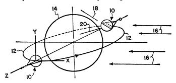
The satellite of the invention is lens shaped. It carries a solar sail which supports a damping weight that cooperates with proper inertia distribution in the body to stabilize the satellite in pitch and roll. Proper mass distribution provides a preferred orientation for the satellite's yawing motion so that the period of oscillation in yaw is twice the orbital period.
