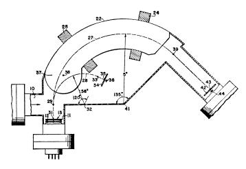
particles to be analyzed and magnetic fields to bend their paths. The amount of curvature depends on the mass of the particles so that particles of different mass arrive at slightly different points on the collector.
