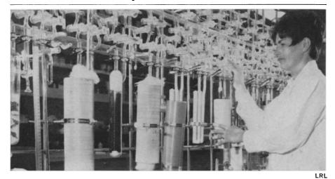
Checking for radioisotopes in samples of gas from a Plowshare program test.
