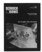
Graphite fibers promise to be an important engineering material of the near future. A graphite yarn is being wound onto a mandrel, or spindle, for application in the aviation or aerospace industries. p. 601. (Photo: HITCO)
