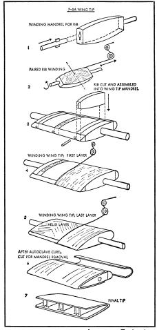
Aerospace Technology Graphite yarn wound into a wing tip.
