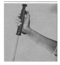
A micropump pipetting device made of polyethylene simplifies pipetting liquids, including corrosive and toxic materials, for the laboratory worker. Pipettes fit easily into the unit, which is equipped with an adjuster that allows the user to preset the stroke of the plunger and dispense precise doses.
