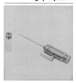
A problem with injecting material into a gas chromatograph, which analyzes minute samples to determine their composition, is the difficulty in getting the same volume of sample into the chromatograph each time. A new submicroliter injector has removed the problem. It offers sample reproducibility, something a conventional injection syringe cannot do since it depends on the manual ability of the operator to repeat his own injecting technique precisely.
