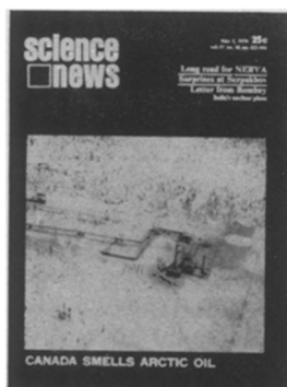
The engineering loop at Inuvik, Canadian Northwest Territories, is testing the movement of hot oil through 48-inch pipe over permafrost. Canada hopes to be a vital link in the transportation if not the production of Arctic oil. See page 442. (Photo: Gene Brush)
