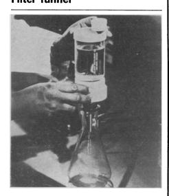
In many areas of drug research, radiological analysis, water pollution investigation and cancer cell studies, the ultrafiltration of liquids is required to separate out extremely small particles or microorganisms. Gelman Instrument Co. has developed a filter funnel system that offers greater protection from outside contamination during the filtration process.
