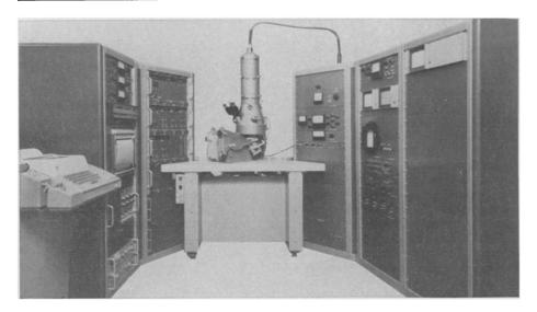
An automated and computer controlled instrument has been devised—the first of its kind, according to Materials Analysis Co.—that combines two analytical instruments in one. The instruments are the electron microprobe and the electron microscope. The result is a combination electron microprobe analyzer and scanning electron microscope that is capable of making complex observations and recordings because of its automated features.
