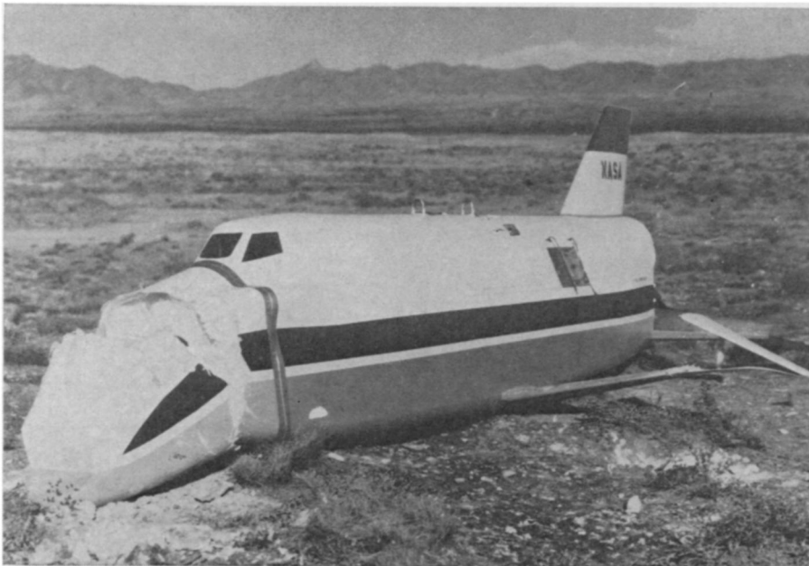
A crushable nose cushions the landing of the mini-shuttle after flight test.
