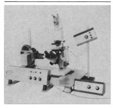
Time-lapse and normal-speed motion pictures can be obtained through either upright or inverted microscopes with the new Sage Instruments, Inc., Model 503. The cinemicrographic apparatus is especially suited for studies of living cells, crystals, corrosive action, or other long-term laboratory in-
