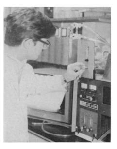
atomic absorption measurement is made using a mercury hollow cathode lamp.
