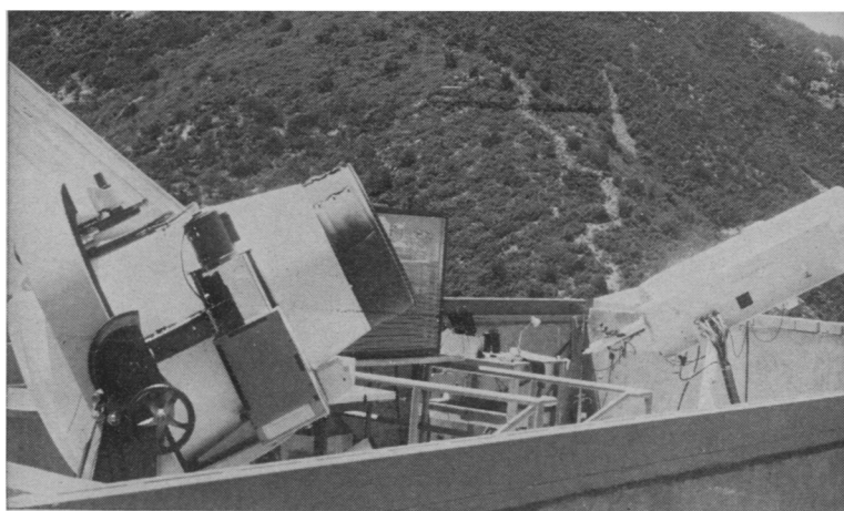
SAO laser-camera pair at Mt. Hopkins Observatory.
