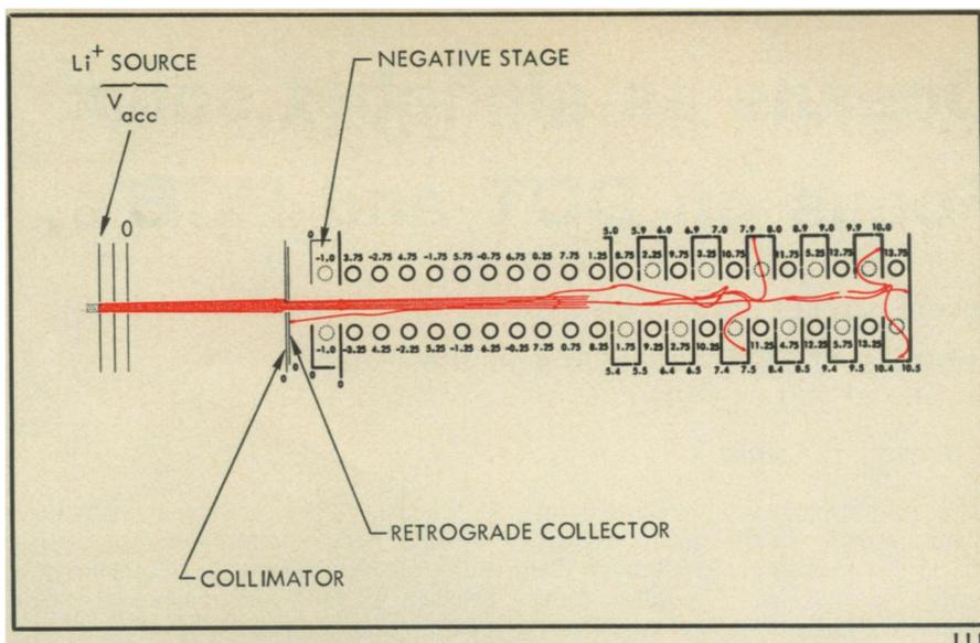
Direct conversion of charged-particle motion to electric current.
