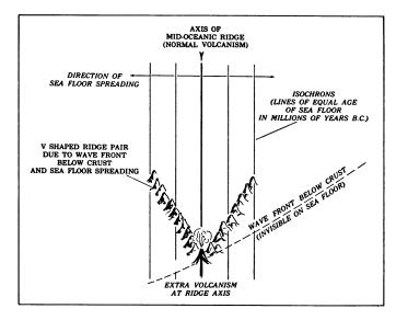
In the Vogt and Johnson model. mantle waves passing under midocean ridges form V-shaped patterns like the wake of a ship.
