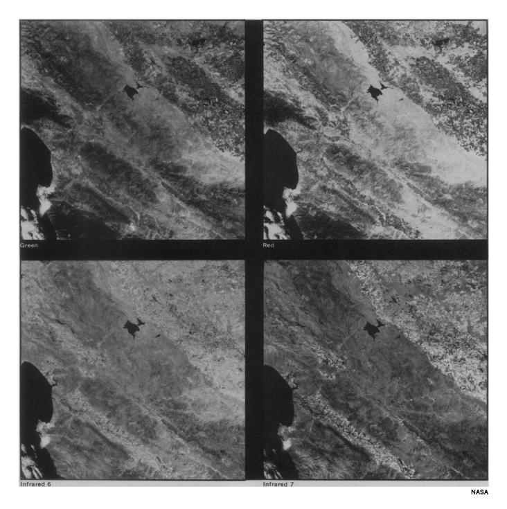
Monterey Bay, Santa Cruz, the Salinas and San Joaquin Valleys and the San Andreas Fault zone were photographed from 900 kilometers July 25 by the multispectral camera aboard ERTS I. Shown are photographs in the green, red and two infrared spectral bands. The infrared bands are in wavelengths 7,000 to 8,000 angstroms and 8,000 to 11,000 angstroms.
