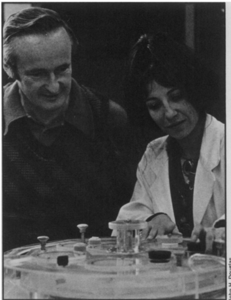
Bassham and Bissell adjust the tissue-culture apparatus they developed to maintain constant nutrient supply and waste removal for cultures of both normal and transformed (cancerlike) cells.
