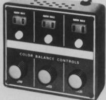
trols, 3 controlled individual SCR circuits, protective isolation transformer, custom plastic housing & complete instructions.
