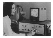
The MINI RAPID-SCAN® from ISI with its guaranteed resolution of 750 Angstroms offers five times the depth of field of the best light microscopes. It fits on a table top and can be operated by anyone. It's proven well-suited for teaching, inspection, process and quality control. Magnification range, 20X to 10,000X; accelerating voltage 10 Kv; TV display. Price \$9,900. Absolutely unique.
