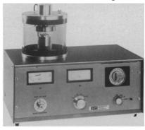
Another ISI value. Model PE-5000 Sputterer-Coater apparatus provides rapid (about 3 min.). uniform coating of even the most irregular specimen surfaces. The diode sputtering technique makes the difference in performance-and price: \$1,695. Especially suited for biological specimens.
