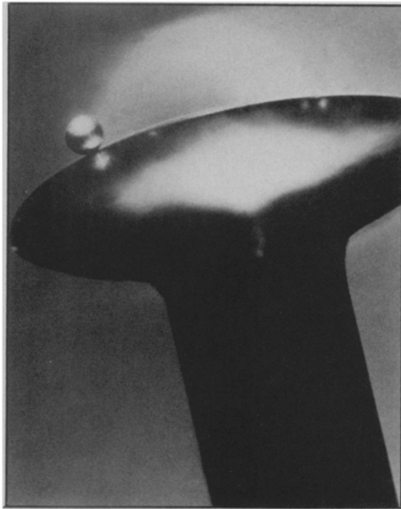
One of the fuel pellets compared to a pinhead.
